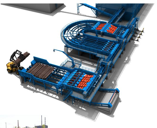
Various conveyor solutions for transporting logs to debarkers, sawlines, chippers, as well as for veneer industry:
